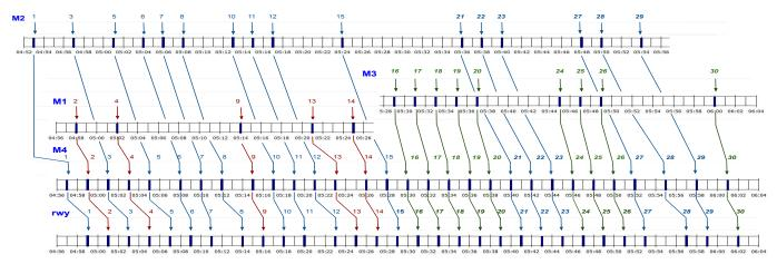
Figure 3. Experiment 1: arrival time schedule at all merge points of the optimized arrival trees for 30 aircraft within Stockholm Arlanda TMA between 4:50 and 6 am on May 16, 2018. Bold italic numbers refer to arrivals on the tree for the second half hour.
