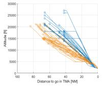
Figure 6. Comparison of the vertical profiles of the actual (orange) vs. optimized CDO-enabled routes (blue) for 30 arrivals within Stockholm Arlanda TMA between 4:50 and 6:02 AM on May 16, 2018.
