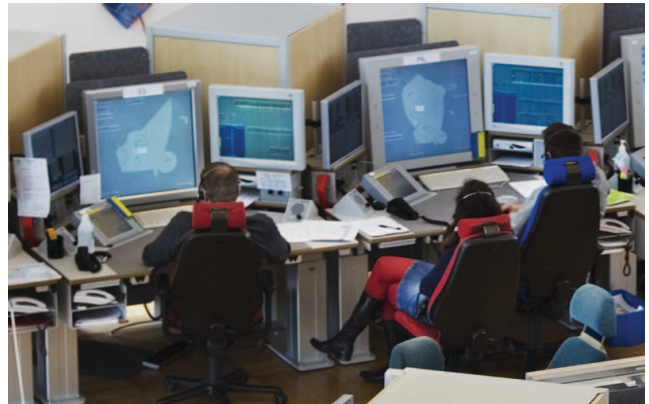
Fig. 1. Air traffic controllers at an Air Traffic Control Centre (ATCC). The image shows two controller working positions with the air situation display (basically a synthetic radar screen) at the central, main screen which is flanked by smaller screens comprising other tools and information displays. Just below and left of the main screen there is a voice communications system touch screen. Press image from www.lfv.se.
