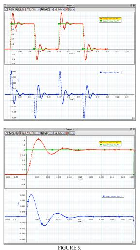
Results from measurement of current through the circuit (lower part) and voltage (upper part) over the whole circuit, and over the capacitor, for  $R=R_{\rm coll},\,L=8.2$  MH and 100  $\mu F.$  The upper and lower graphs have different time scaling on the X-axis.
