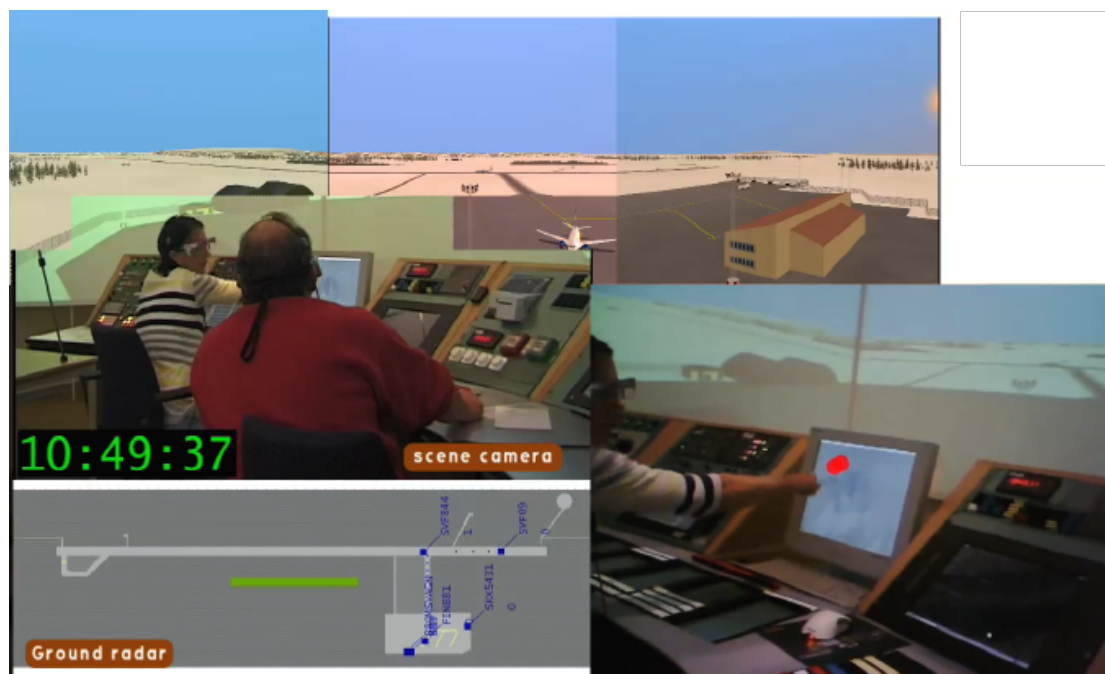
Figure 9. Synchronised video sources for recording X, at 10:49:37. ATC tower room and simulated outside view (top mid), ground radar (middle, not available to the ATC, added to show aircraft positions more clearly), ATC eye-point-of-gaze recording (for the ATC on the right).
