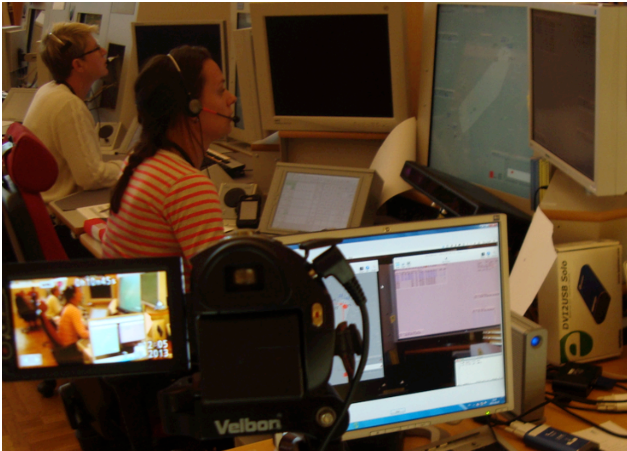
Figure 5. Each scenario was video recorded, showing both planner and executive, as well as the recorded ATC screens and the gaze plot recording (small screen next to the video camera in front in the photo) simultaneously.
