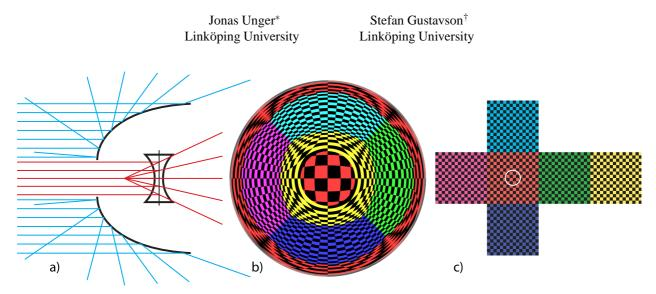
Figure 1: a) A principal sketch of the mirror and lens setup, with reflected and refracted rays for the parallel projection case. b) An image of a checkered environment map, as displayed in c), as projected by the setup. The field of view of the central lens is about  $30^\circ$ , represented by the white circle in the cube map.
