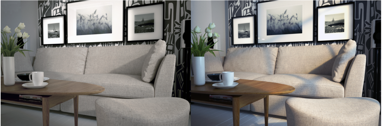
Figure 1: Left: synthetic scene rendered with traditional image based lighting, using a single representative light probe for illumination. Right: the same scene, rendered with scene data extracted from tens of thousands of light probes to accurately capture the complex spatial variation in the illumination.
