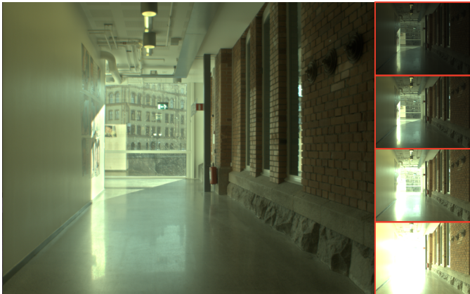
Figure 10: Top: An overview of our experimental HDR video camera. Bottom: a full resolution locally tone mapped frame from a video sequence captured with the HDR video camera. The image is reconstructed from four 4 Mpixel sensors at 26 fps. Bottom-right: Four gamma mapped images 2 f-stops apart from the same HDR-image.
