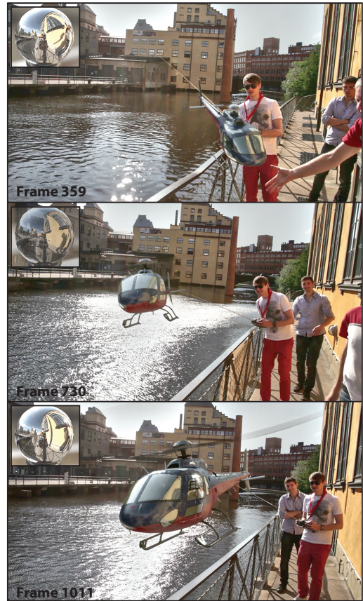
Fig. 4. Three frames from a video sequence of a virtual helicopter rendered using temporal IBL. The lighting measurement used in each frame is shown in the left upper corner.
