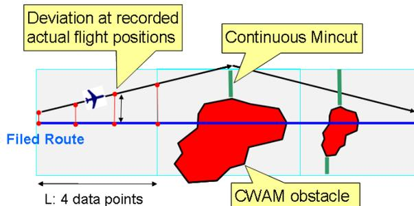
**Figure 6:** Illustration of methodology for measuring deviation and mincut.
