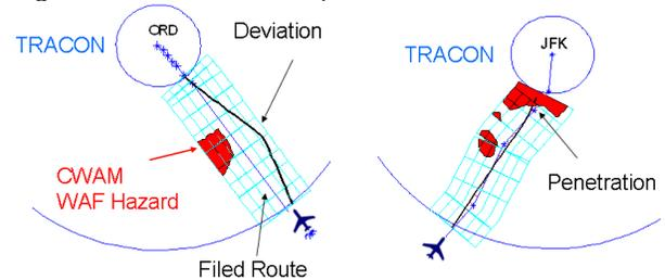
Figure 12: Examples of CWAM weather hazard deviation (left) and weather hazard penetration (right).
