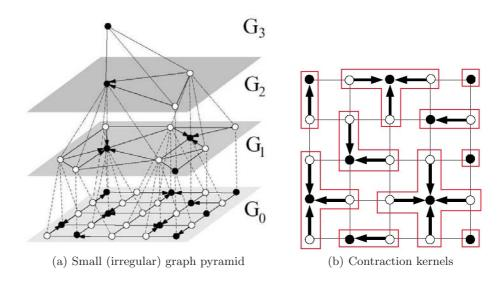
Fig. 1. Graph pyramid and contraction kernels are based on a  $5 \times 5$  pixel image (images were taken from [5] and [6]). Directed edges represent the contraction processes, white nodes are collapsed in the next upper level, and dotted edges between the levels symbolize together with the connected nodes all contraction kernels.
