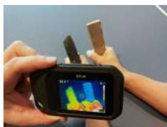
Figure 1. Respective heat conducting and insulating properties of metal and wood demonstrated by the image on the thermal camera.
