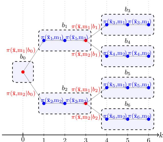
Fig. Approximation of a scenario tree considering one other vehicle with two actions.
