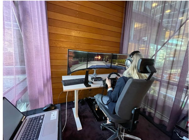
Figure 1: Experiment setup. The arrow seen in the top of the middle screen is an example of one of the navigation instructions provided along the route. The hood of the virtual ego vehicle can be seen in the bottom of the middle- and right screens.
