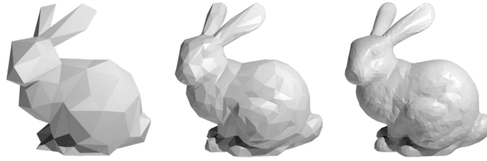
Figure 2.16: A range of predefined meshes with increasing resolution. Dynamic level of detail algorithms are used to choose the most suitable mesh for rendering
