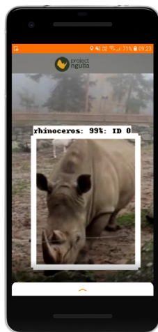
Figure 4.8: A TFLite model can be integrated in an Android/iOS App for demonstration of the detection model.
